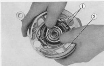
Fig. 4.86 Disassembling brake shoes
