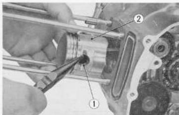
Fig. 3.49 Removing the piston pin
