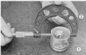
Fig. 3.52 Measuring piston skirt diameter
