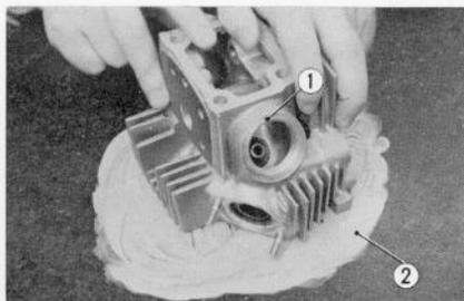
Fig. 3.18 Checking cylinder head warpage
